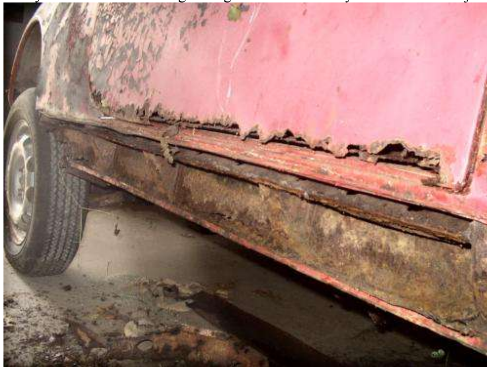
The gutted sill area
