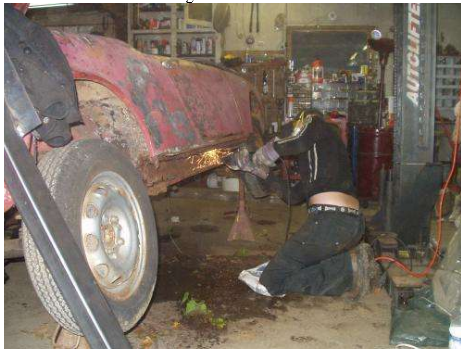
Cleaning out the inner sill
